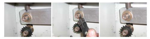
13. Remove all four of the roller pressure adjustment knobs located on the top of the side panel use a ¼" allen wrench to remove these screws keep track of how many turns it takes to remove them when reinstalling them in step 49 you will want to put them back to this position.
