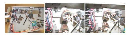
18. Remove the brushes. Loosen the set screw that holds in the brush holders partially remove the brush holder then pull out the wires from the brush holders (they pull out do not de-solder these). (Unlike step 10. the brushes will not spring out of the front of the holder they are trapped).
