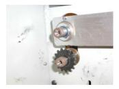
44. Install the slip ring on the upper roller shaft (similar to step 33.), before tightening the set screw make sure that the rollers are properly aligned and the set screw is on the flat as in step 32.
