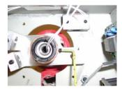
45. Solder the wires to the slip ring, (similar to step 36.) be very careful as the wires are very fine (28 AWG) and quite fragile, If these wires must be stripped use painstaking care to make sure these are not damaged, hold the wire back with your fingers when stripping to relieve strain on the wire. These wires are not polarity sensitive and may be attached to either post. If these wires are broken it will render the roller in operable
