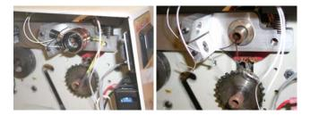
12. Remove the snap ring on the upper rear roller discard the snap ring, do not reuse the snap ring. If there are any spacers on the shaft, these must be put back in step 43.
