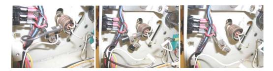
23. Remove the slip ring using a 5/64 allen wrench (similar to step 11).
