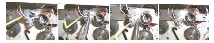
11. Loosen the set screw holding the slip ring onto the roller and remove the slip ring. You may rotate the rollers to get a better angle at the screw if necessary.
