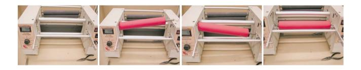
29. Insert the upper laminating roller following the sequence in step 20 in reverse. It may necessary to align the hole in the swing arm by pushing up on the swing arm
