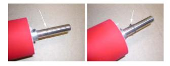
32. Align the top roller to the bottom roller by sliding the bottom roller to the left so that the snap ring is snug against the side panel. Then move the top roller so that the edge of the top roller is aligned with the edge of the bottom roller. Then align the rear roller set using the same procedure.
