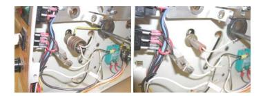
24. Remove the snap ring holding in the lower roller then remove the bushing and any spacer (similar to step 12.)
