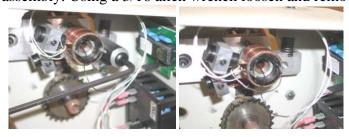
10. Remove both of the sensor wires brushes and brush holders. Using a 5/64 allen wrench loosen the set screw, slide the brush holder back then pull the connector with the wire away from the front of the holder, remove the brush from the front of the holder, remove the holder. These brushes are spring loaded and may spring out of the brush holder use a needle nose pliers to carefully remove them.
