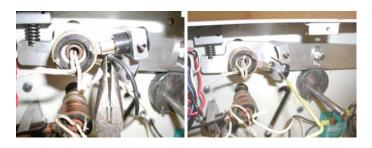
19. Remove the slip ring using a 9/64 allen wrench (similar to step 11.) If the screw is severely corroded and the socket becomes stripped out use a needle nose locking pliers or small locking pliers to remove it, then replace the screw.
