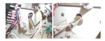
31. Install a **NEW** snap ring into the groove on the lower roller, make sure not to stretch the snap ring to far, make sure that the snap ring is completely in the groove. **If the snap ring is damaged at all during installation, make sure to replace it.** Illustration shows the proper position of the snap ring, do not install the snap ring before the roller is in the machine (the pictures below are for reference to the groove)
