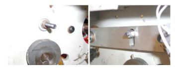
43. Install the snap ring and any spacers that were removed on the upper rear roller in step 12. Make sure snap ring is in its groove as shown in step 31
