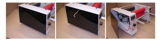
2. Remove roller-gapping handle by turning counterclockwise. This handle is located on the right side of the machine and it may require some one to hold the roller-gapping cam located under the swing in the left side panel with a large pliers. After, make sure the rollers are in the down position.
