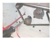
51. Install the rubbing pad assembly. Apply a liberal amount of supplied silicone lubricant to inside of the felt pad as shown then a thin film on the top of the felt. Tighten the rubbing pad while applying pressure from the bottom of the spring. Use only enough pressure to slightly deflect the spring as shown in the picture
